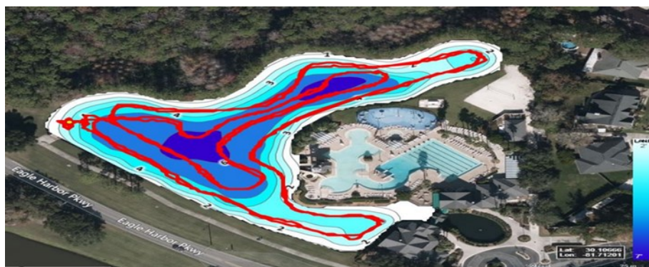
Fig. 5 C-Map BioBase tracks and bathymetry output as collected by ADAPT™.
